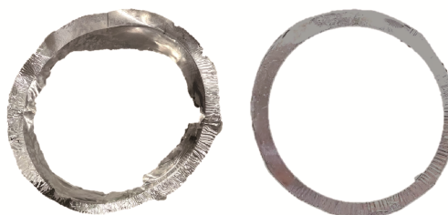
(b) 软铝膜片(左)与硬铝膜片(右)破裂图 (b) Rupture diagram of soft (left) and hard (right) aluminum diaphragms
