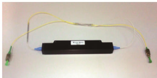
(c) 光纤耦合波长标准器 (c) Fiber-coupled wavelength etalon
