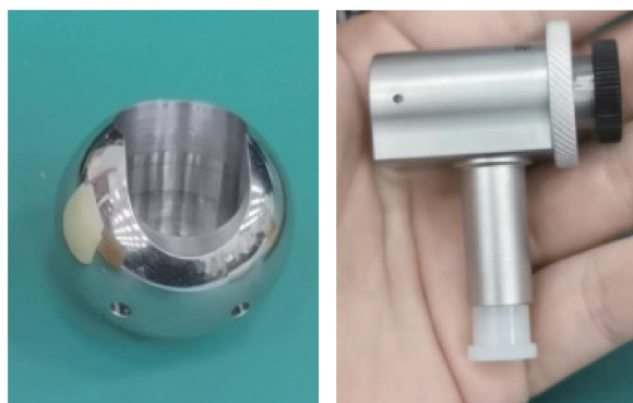
(a) 球形准直器球体示意图 (a) Schematic diagram of the spherical body of spherical collimator
