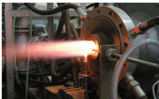
图 12 航空工业计量所的热校准风洞 Fig.12 Hot calibration wind tunnel of AVIC Changcheng Institute of Metrology & Measurement
